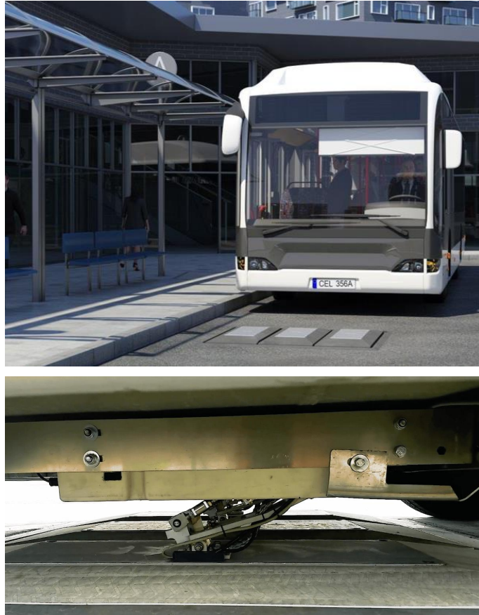
In-line ground based static charging (Alstom SRS)
