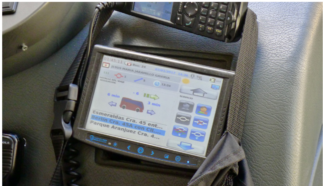
Figure 13. On-board console for managing bus headways.
