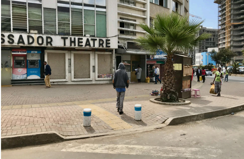
Figure 28. Bollards can help prevent parking encroachments on pedestrian spaces: Addis Ababa.
