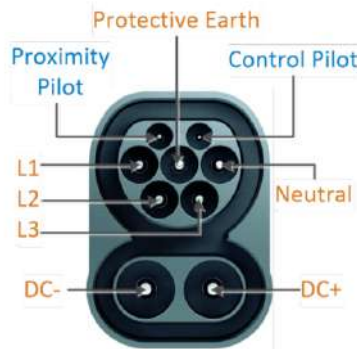
Figure 3.11: Connection pins in CCS2 connector
