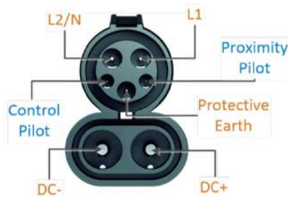
Figure 3.10: Connection pins in CCS1 connector
