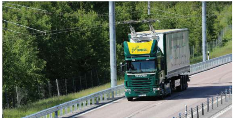
Figure 8.12: Overhead lines in use for road electrification
