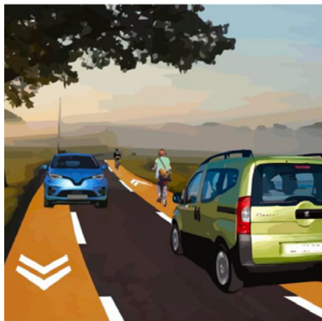
Operating principle of a roadway without centrelines (Kernfahrbahn)
