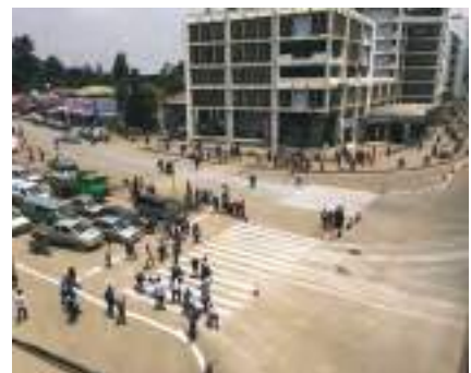
Addis Ababa, Ethiopia. An interim transformation showcasing the principles such as tightening the corner radii, adding appropriate intersection markings and reducing crossing distances.
