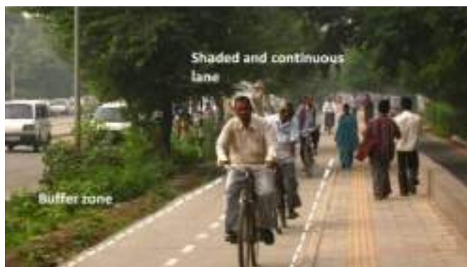
Figure 3.41: Walking and cycling facilities with buffer zone.
