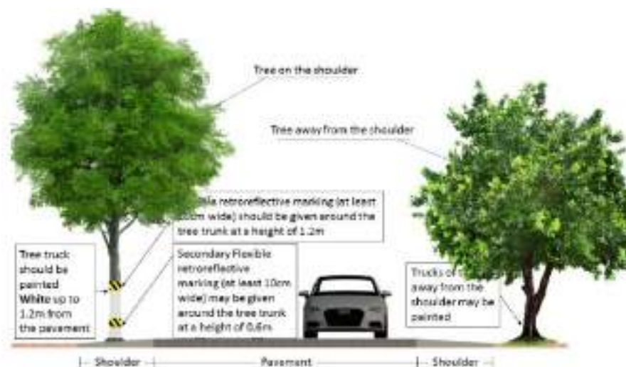
Figure 5.79: Illustration on delineation of trees as a last resort treatment. Delineating hazards may be used in combination of other treatments, including reduction in speeds and protection by safety barriers.
