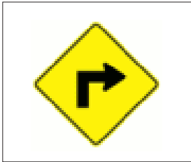
Approaching turn may be hazardous without first reducing speed
