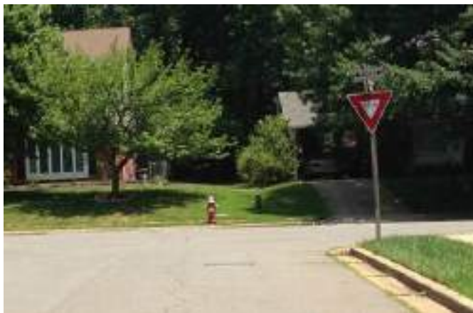
Figure 6.3: Yield signs being used as intersection control.
