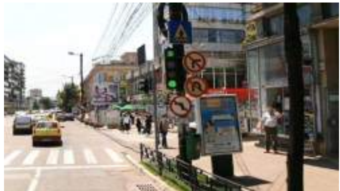
Figure 5.162: Overuse of signs is distracting.
