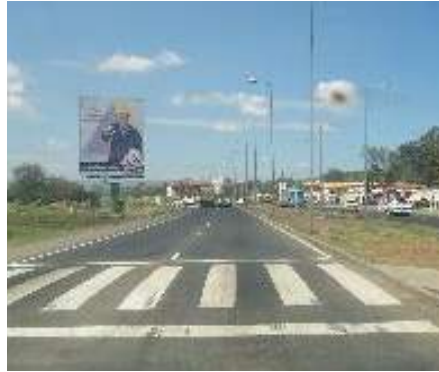
Figure 4.21: Raised crossing to slow approach speeds—Kenya.
