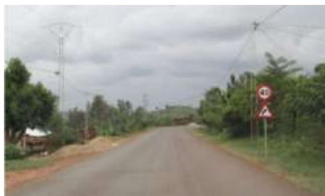
Figure 5.26: Advance curve warning and speed sign.
