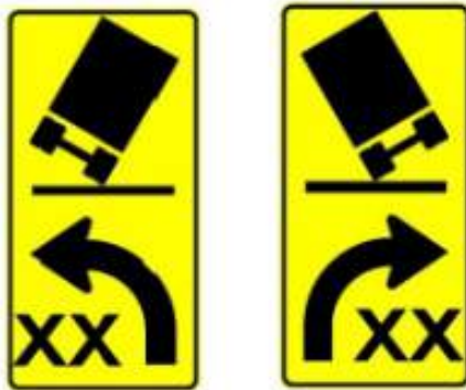
Figure 6.55: Truck tilting warning signs with advisory speed.
