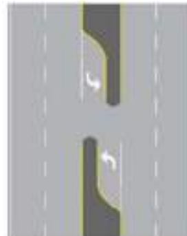
Figure 5.106: Median crossover, opening, with left/right turn bay.
