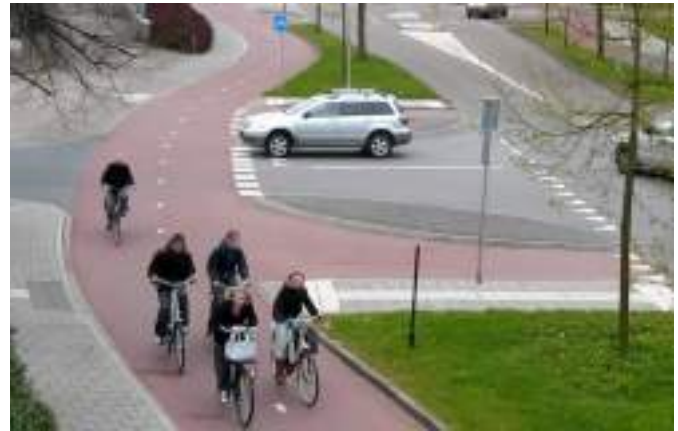
Figure 4.43: Right-of-way intersection (for cyclists)—Holland.
