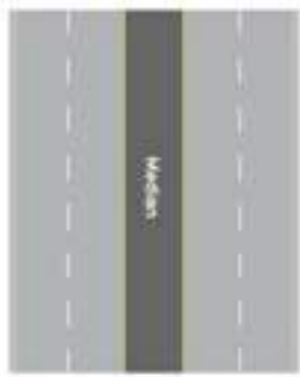
Figure 5.104: Full median with no opening.
