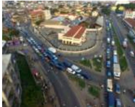
Figure 6.62: Poor delineated slip lane in Ghana.
