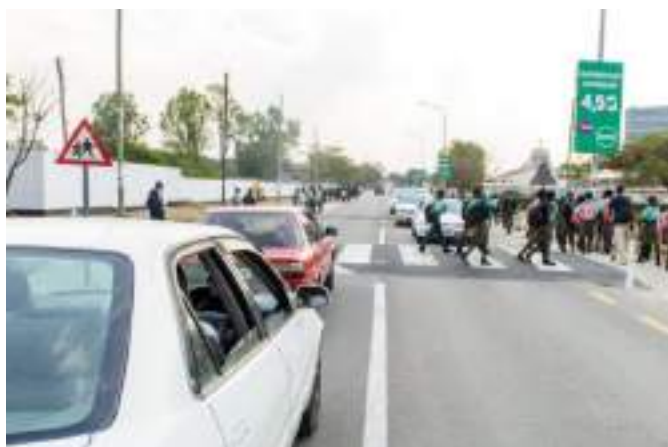
Figure 3.13: School children are protected by an elevated zebra crossing which is a traffic calming feature in itself.
