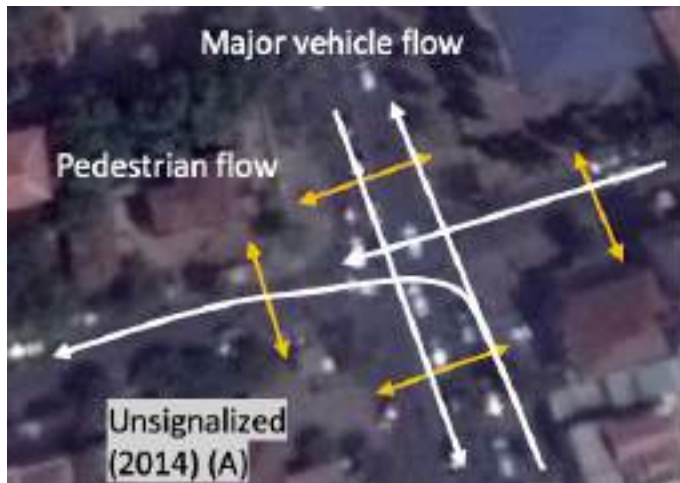
Figure 6.29: Traffic flows at unsignalized intersection without pedestrian crossings in Phnom Penh, Cambodia.
