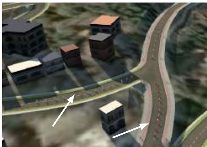
Figure 5.52: Flexible posts improving visibility of median at intersection.
