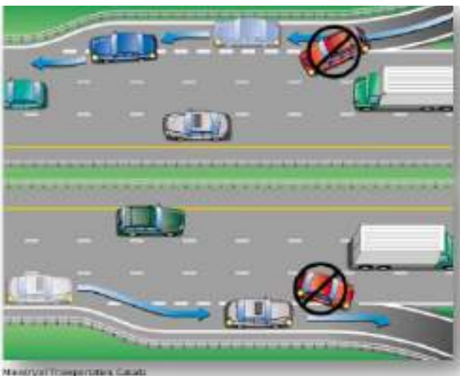
Figure 6.77: Illustration of acceleration and deceleration lanes.
