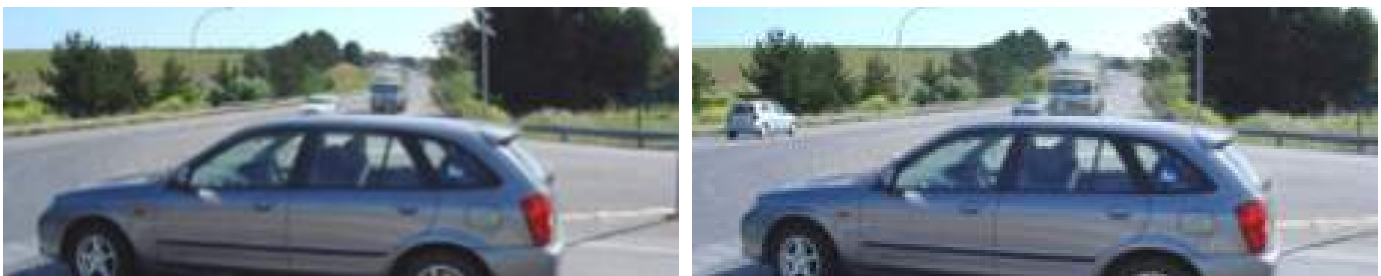
Figure 6.59: Shadowing effects (dynamic visual obstruction)—a large vehicle in the slip lane hiding a vehicle in the through lane.
