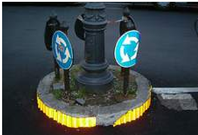
Figure 6.47: Example of mini-roundabout with reflection in Italy.
