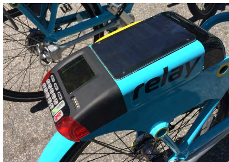
In Atlanta, Relay bikeshare bikes are equipped with a solar-powered keypad and RFID card reader, either of which can be used to unlock the bike. Source: Alta Planning + Design (Flickr CC)
